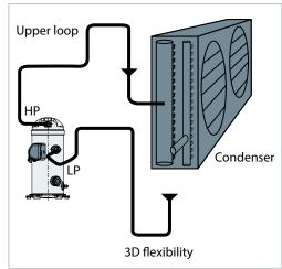
3. Piping should be designed with adequate three-dimensional flexibility to avoid excess vibration. It should not be in contact with the surrounding structure, unless a proper tubing mount has been installed.
