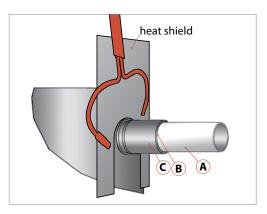
Before eventual un-brazing of the compressor or any system component, the refrigerant charge must be removed.
