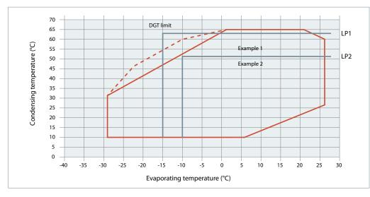
Example 1 (R410A, SH = 6K / 10.8°F) LP switch setting: LP1 = 3.3 bar (g) / 48 psig (-15.5°C / 4.1°F) HP switch setting: HP1 = 38 bar (g) / 551 psig (62°C / 143.6°F) Risk of operation beyond the application envelope. DGT protection required.
