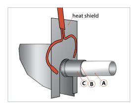
Before eventual un-brazing of the compressor or any system component, the refrigerant charge must be removed.
