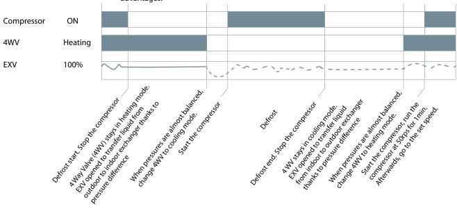
\* EXV Opening degree and time have to be set to keep a minimum pressure for 4 way valve moving.
